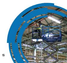
The quiet, electrically-powered Genie® GSTM-2632 slab scissor lifts are excellent for indoor and outdoor construction, maintenance and installation applications on firm, level surfaces.
